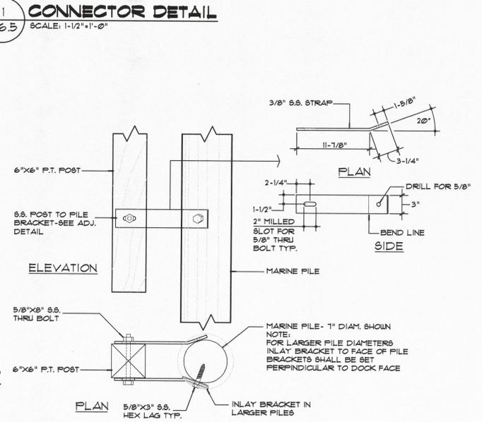
**POST TO PILE CONNECTOR BRACE DETAIL**
