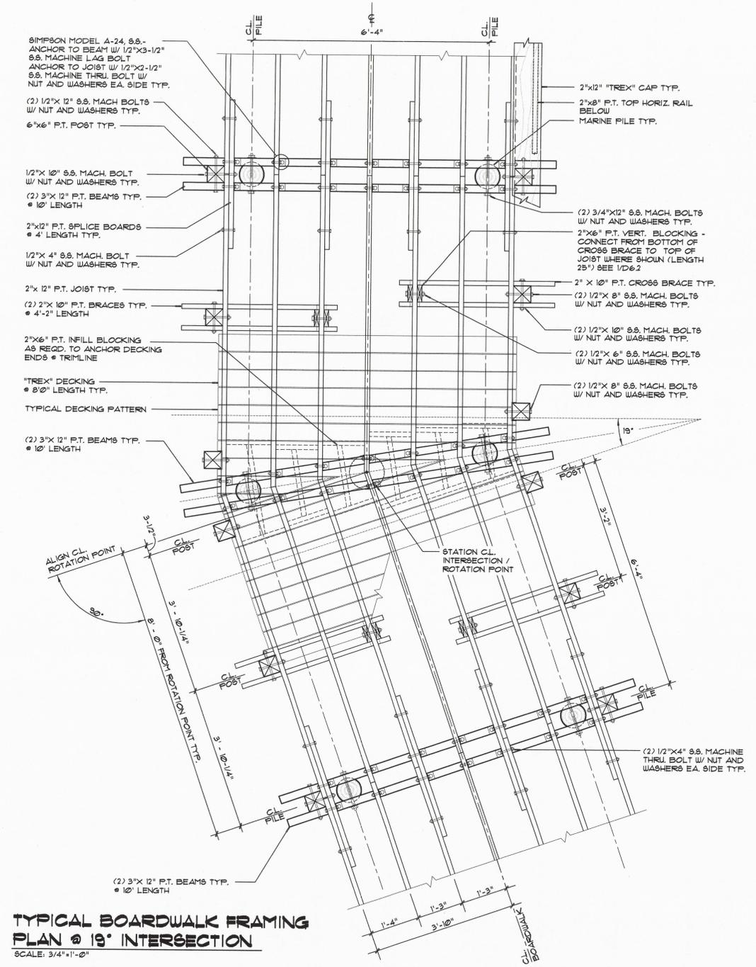
**TYPICAL BOARDWALK FRAMING PLAN @ 19° INTERSECTION**
