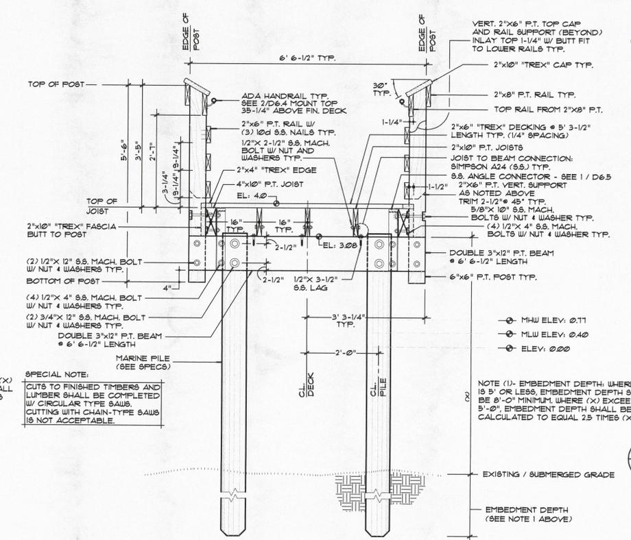
**TYPICAL FINGER DOCK BOARDWALK SECTION W/ HANDRAIL**
