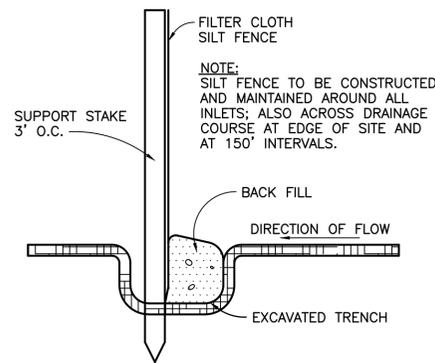
**TYPE III SILT FENCE DETAIL**
