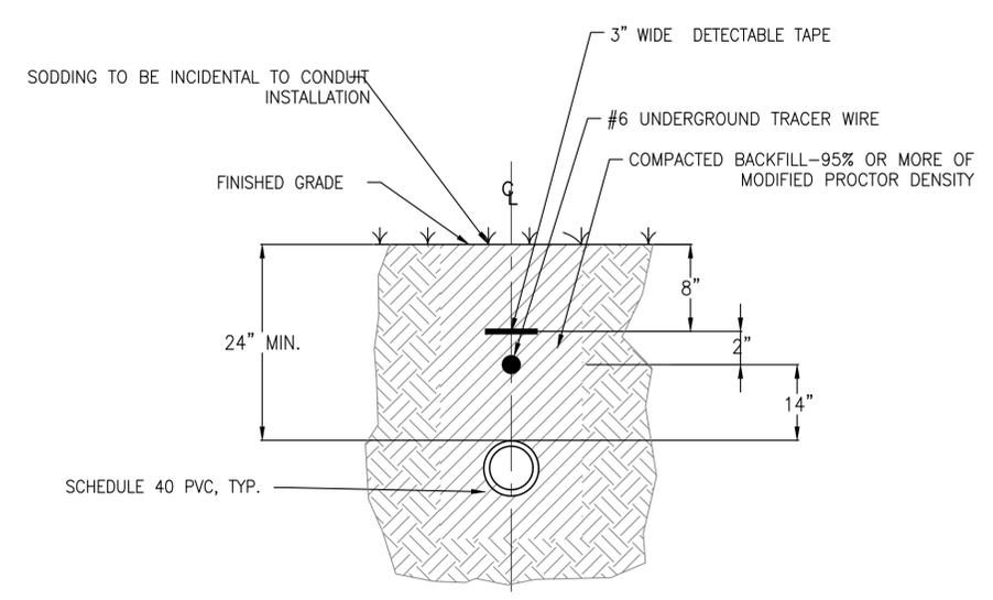
4 COMMUNICATION DUCT CROSS SECTION
