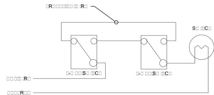
5 3 WAY SWITCH WIRING INSTALLATION DETAIL
