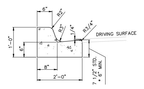
\* NOTE: WHEN USED ON HIGH SIDE OF ROADWAYS, THE CROSS SLOPE OF THE GUTTER SHALL MATCH THE CROSS SLOPE OF THE ADJACENT PAVEMENT. THE THICKNESS OF THE LIP SHALL BE 6", UNLESS OTHERWISE SHOWN
