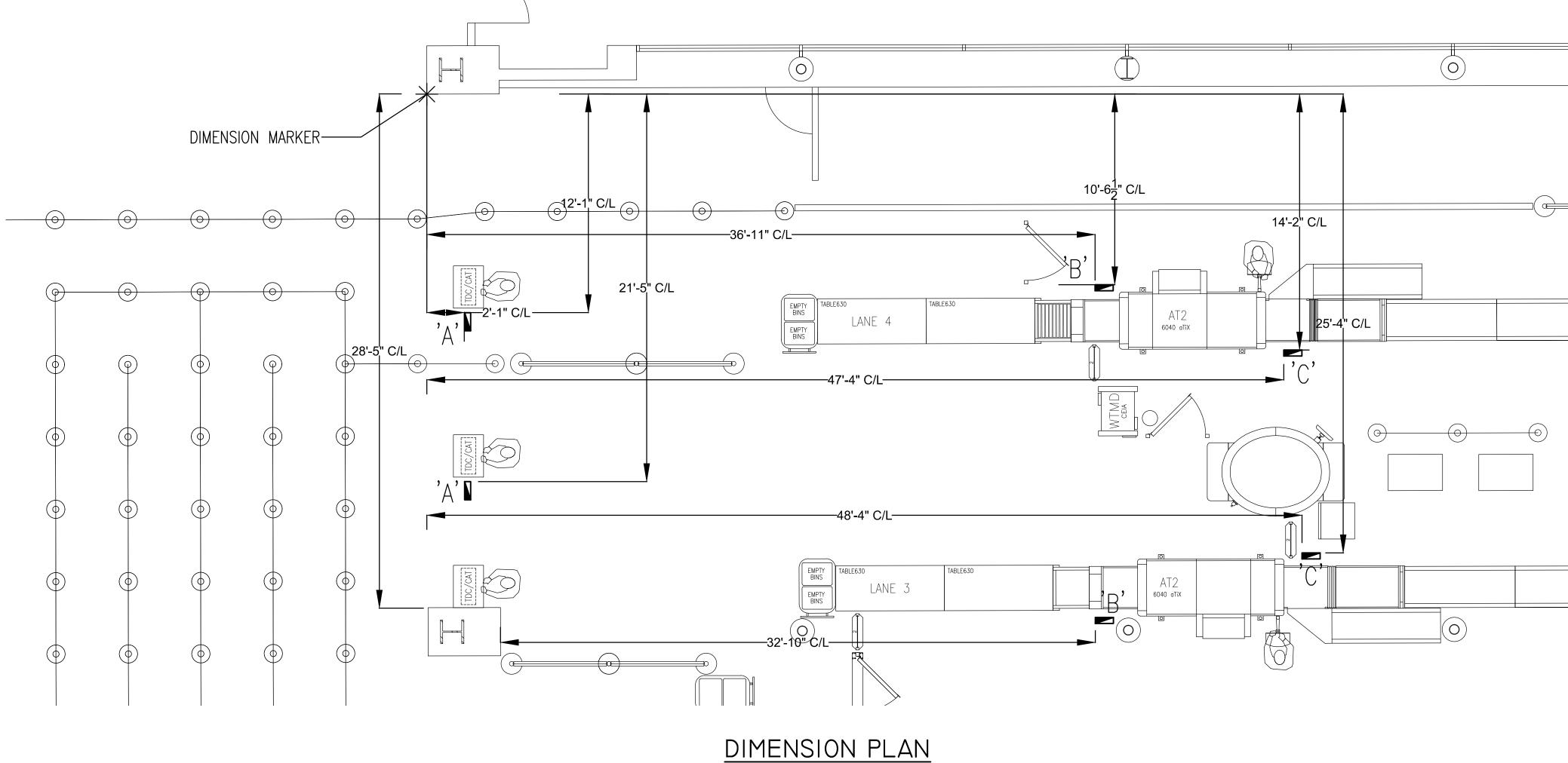
DIMENSIONS SHOWN ARE APPROXIMATE AND TO BE FINALIZED WITH BOTH TSA AND VPS PRIOR TO INSTALLATION.
