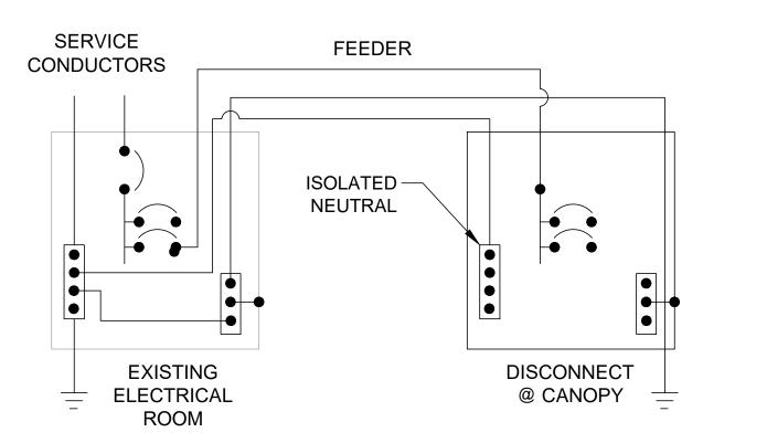
GROUNDING AND BONDING INSTALLATION DETAIL
